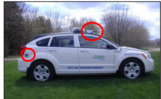
Parking enforcement vehicle with cameras highlighted
